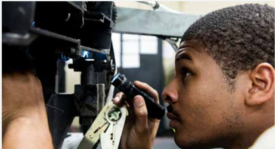
Air Force Senior Airman James Jennings, 23rd Maintenance Squadron, performs an inspection on a 30mm GAU-8 Avenger Gatling-style gun system at Moody Air Force Base, Georgia. The armament shop performs maintenance using DLA-supplied parts to provide aircrews with safe, reliable weapons systems.
